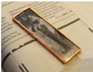
Before burnishing - edges not well adhered
