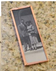
After burnishing - see how flat copper tape looks
